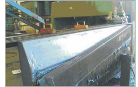
Portacut with 1 torch (standard) cutting a 300mm slab
